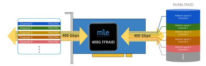
Now, you can transfer bulky data from multiple sensors to a RAID of NVMe SSDs at speeds up to 400 Gbps. MLE's Fast FPGA RAID implements a channel-based architecture, supports data-in-motion pre- and post-processing and is highly scalable with regards to bandwidth and recording capacity. Multiple systems can further be cascaded via high-accuracy IEEE time-synchronization for faster or deeper recording.
