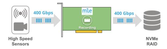
Communication from a high-speed data source can be transported to a data sink while this data is also recorded at-speed.
