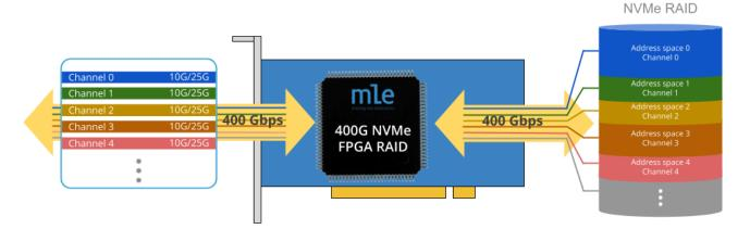
Now, you can transfer bulky data from multiple sensors to a RAID of NVMe SSDs at speeds up to 400 Gbps. MLE's NVMe FPGA RAID implements a channel-based architecture, supports data-in-motion pre- and post-processing and is highly scalable with regards to bandwidth and recording capacity. Multiple systems can further be cascaded via high-accuracy IEEE time-synchronization for faster or deeper recording.
