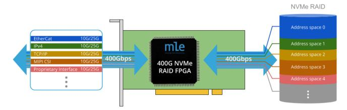
Now, you can transfer bulky data from multiple sensors to a RAID of NVMe SSDs at speeds up to 400 Gbps. MLE's NVMe RAID implements a channel-based architecture, supports data-in-motion pre- and post-processing and is highly scalable with regards to bandwidth and recording capacity. Multiple systems can further be cascaded via high-accuracy IEEE time-synchronization for faster or deeper recording.
