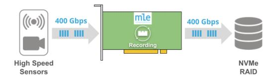
Communication from a high-speed data source can be transported to a data sink while this data is also recorded at-speed.
